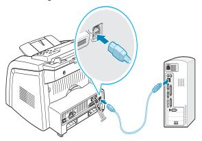
If you want to use a parallel printer cable, purchase only IEEE 1284 compliant parallel cable and connect it to the parallel connector on your machine.
